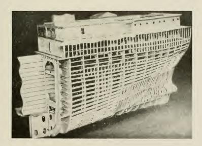
Fig. **67** Framework of a motor freightship.
